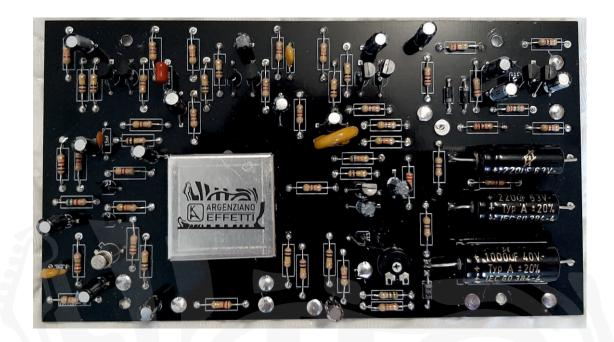
Populate your PCB starting from resistors, trimmer, capacitors, transistors and at the end LDR's and bulb.
